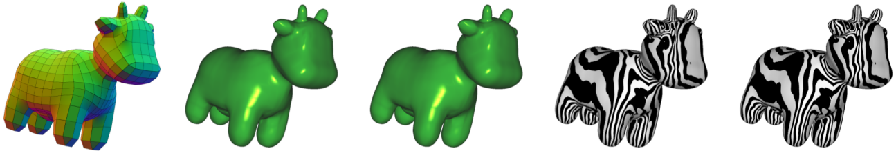
Figure 1: From left to right: The input mesh (Spot; 56 triangles, 634 quads, 40 pentagons, and 4 hexagons), shading on Gregory S-patches, shading on Gregory generalised Bézier patches, reflection lines on Gregory S-patches, and reflection lines on Gregory generalised Bézier patches.
